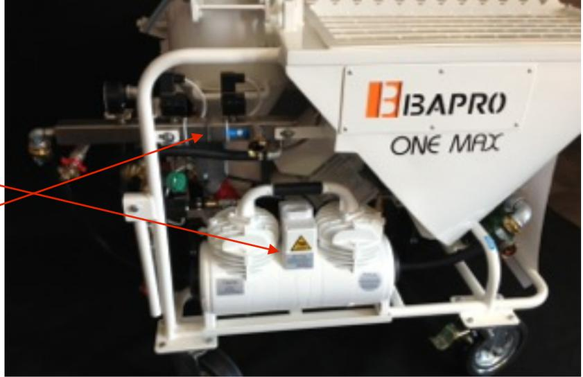
**Water pump type 50M** ensures the continuity of work to stabilize the water pressure and provide the best consistency of the mortar.
